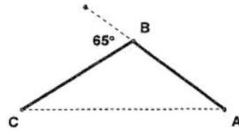
11. A triangular parcel of ground has sides with lengths 725 feet, 650 feet, and 575 feet. Find the measure of the largest angle on this lot.
